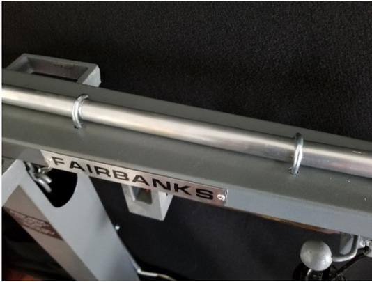
The ParaSCALE Lite-SL is easy to mount. Simple drill 4 holes in the top arm of the scale and secure with the U-Bolts provided, place the proximity trigger in position, and then align the explosion proof sensor with the balance arm, centered in the indicator bracket. Connect 120 vac as per the instructions, and pump discharge hose to the ½" solenoid and it's ready to go! Installations typically take less than 30 minutes
