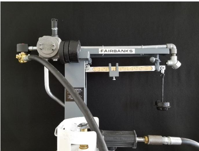
Installation and calibration take about 30 minutes. Does not affect scale operation. Mounts to standard Fairbanks filling scales (more applications coming).
