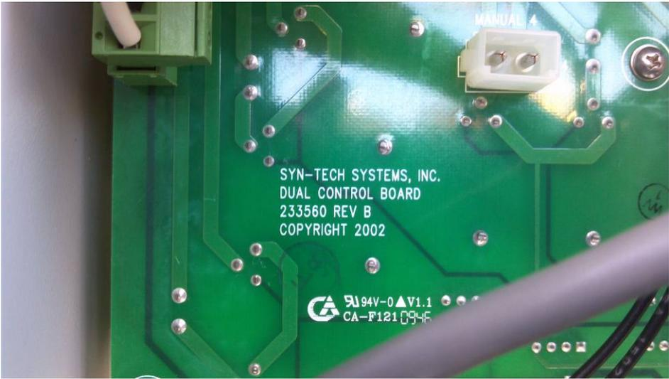
ILLUSTRATION 4: Correct Pump Control Board, FuelMaster Part Number “STS#233560, RevB, Dual Control Board”. (This replaces Standard high voltage/amperage pump control board, if so equipped)
