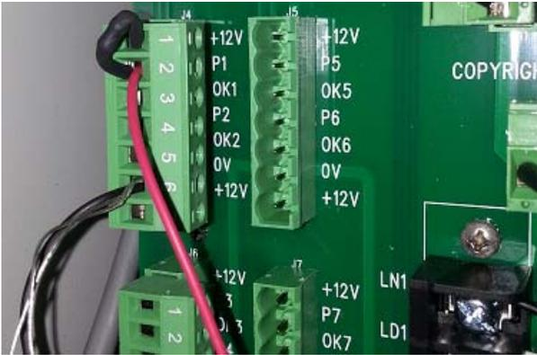
ILLUSTRATION 5 – PARAFOUR Dispenser Pulser circuit wiring. PARAFOUR RED wire (Pulser +) connected to P1. PARAFOUR BLACK wire (Pulser -) connected to “0V”. 330 ohm, ½ watt resistor between “12V” and “P1”. NOTE: The BLUE wire in the illustration should be BLACK. (Photo taken from field installation).
