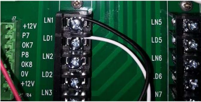
ILLUSTRATION 1: Dispenser Authorize connections from Dispenser to FMU (Connections shown at FMU). Connect to “LN1” and “LD1 (Photo taken from field installation).
