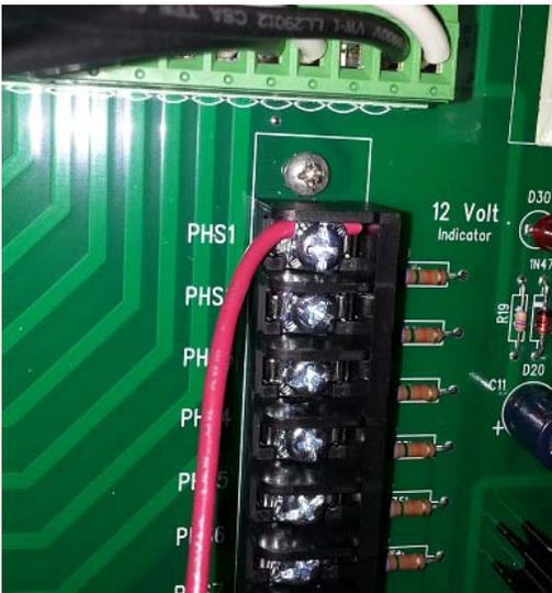
ILLUSTRATION 2: Dispenser “in-Use” or “Pump Handle Signal” from Dispenser to FMU (Connections shown at FMU). Connect to “PHS1”. Note that wire indicated in the photo is Orange, however the actual Pump handle Signal wire from the dispenser is RED. (Photo taken from field installation).
